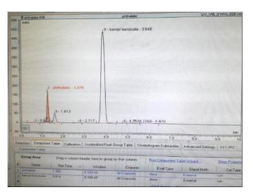
**Figure (1):** Chromatogram of spiked urine sample containing 4µg/ml of monobutylphthalate (MBP) and benzyl benzoate (internal standard), concentrations 10µ l.
