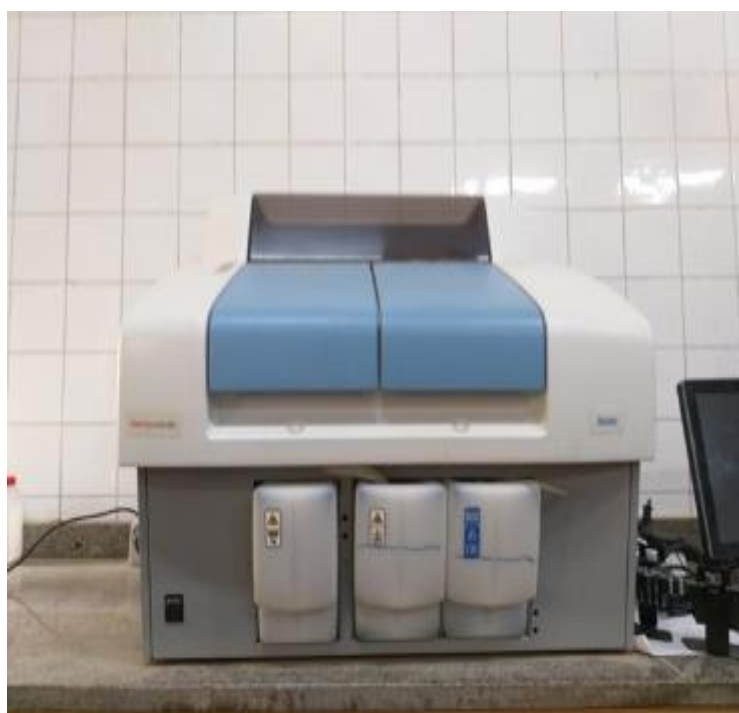
Figure (2): Indiko thermoscientific fully automated urine enzyme immunoassay. (Thermo Scientific Indiko Chemistry Analyzer manual, 2013).
