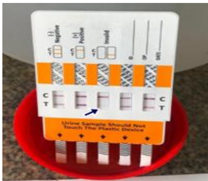
Figure (1): Immunoassay test strip interpretation the test is positive for cannabis (one line at the C region), as shown by the black arrow, while it is negative for the rest of the drugs (two lines, one at the C and the other at the T regions).
