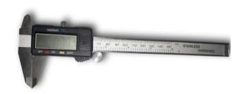
Figure (1): Digital Vernier caliper
