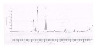
Figure 8: Gas Chromatography-Head Space chromatogram showing positive result for ethanol in exhibit (Blood) at 3.9 min (Retention time)
